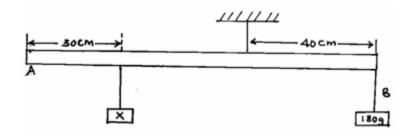
The rule is 1m long and weighs 1.8N. Calculate the weight of the block X. (3mks)
