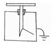
Given a dry glass rod and silk cloth, explain how you would determine the type of charge on the electroscope. (2mks)
