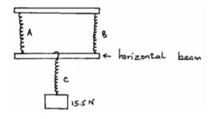
If the weight of the horizontal beam is 0.5N, determine the extension of each spring given that 4N cause an extension of 1cm when using one spring. (3mks)
